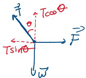
$$\begin{aligned} F &= T \sin \theta \\ mg &= T \cos \theta \\ F &= mg \tan \theta \end{aligned}$$
