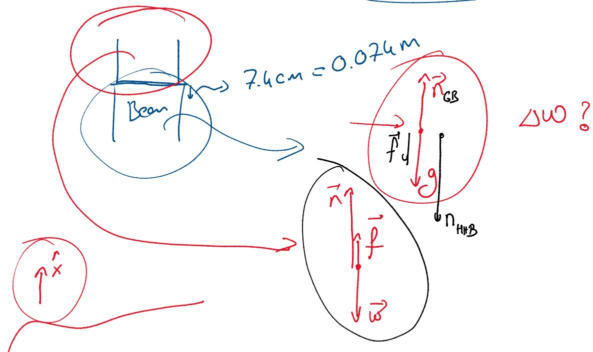
$$(\vec{n} + \vec{f} - \vec{\omega}) \cdot 0.074 \text{ m} = 0 - \underbrace{\frac{1}{2} 200 \text{ kg}}_{= 5700} \underbrace{(7.55 \text{ m/s})^2}_{= 5700}$$
